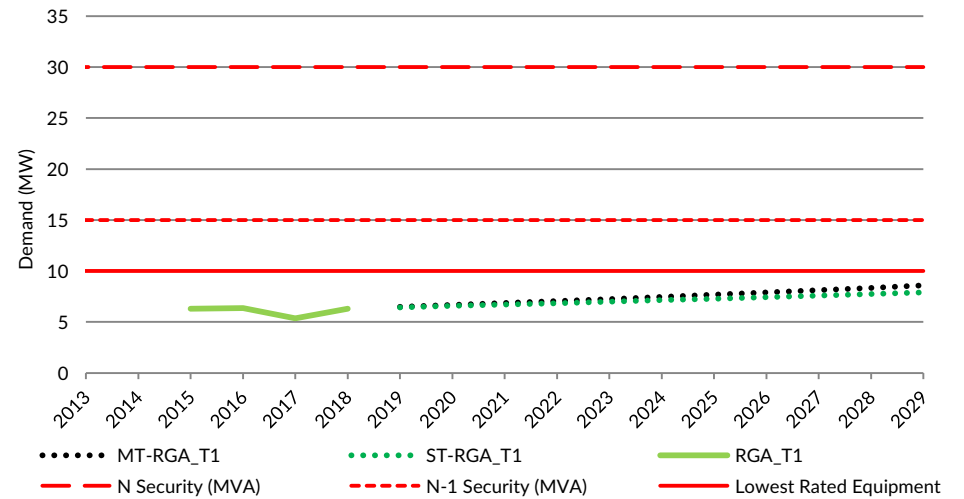
Figure 5.29 Rangitata 1 zone substation demand forecast
