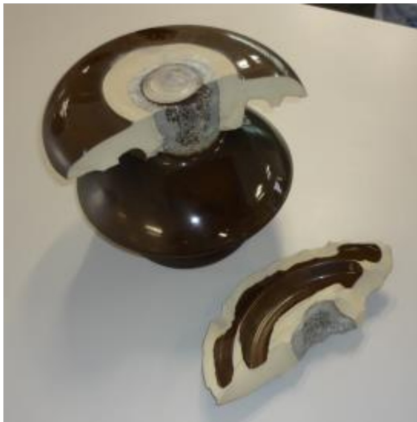
Photograph 9: Example of two piece 33 kV clamp top insulator failure
