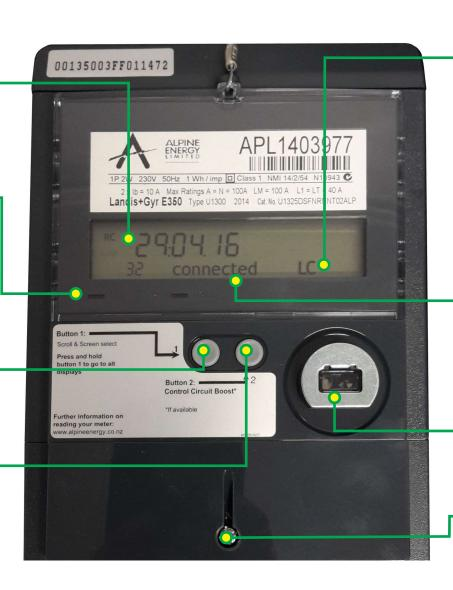
LC/LC1 indicates there is a controlled load on this meter, usually only for appliances that run overnight or in off-peak times i.e. hot water, night store or underfloor heating.
